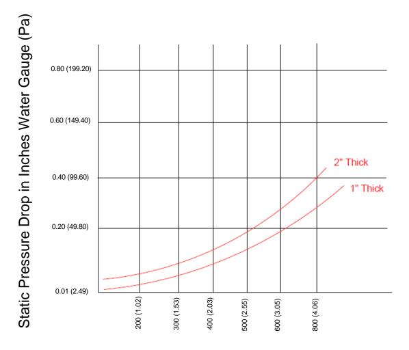
Air Velocity in Feet Per Minute (Meters Per Second)
